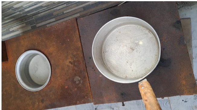
Figure 6: Water Boiling Test on Forced Draft Stove
