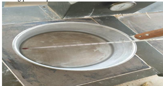
Figure 5: Water Boiling Test on Natural Draft Stove
