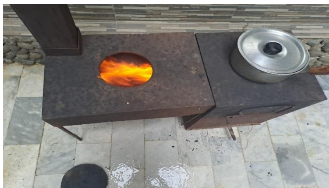
Figure 3: Forced Draft Stove with Amplified Flames Inside Secondary Plate Chamber.
